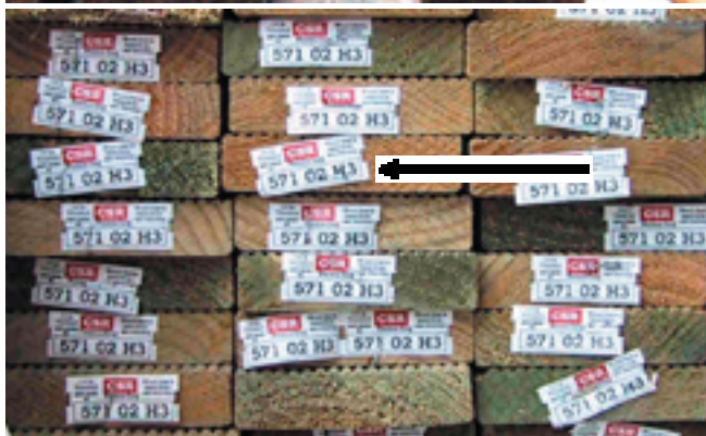
Two types of branding or marking to demonstrate that the timber has been treated in accordance with AS 1604-2000 (Photographs courtesy Harry Greaves)
